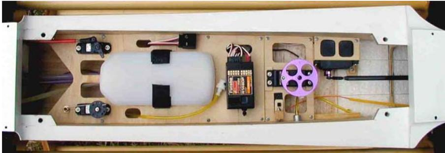
With the fuel tank mounted in what would normally be the radio bay, you need to pay extra special attention to ensure the silicone pipes can't come off when filling the tank (don't ask me how I know!!). I now solder a small wire loop onto the end of brass tubes exiting the fuel tank and secure the silicone tubes with spring clips.
