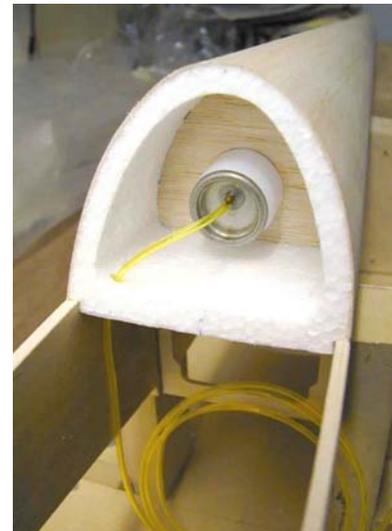
*Spirit Top Deck. Note the retract air tank glued to two 1.5mm balsa formers before mounting.*
