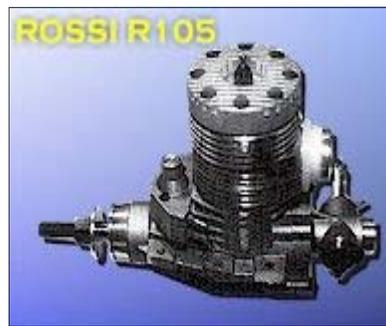
The engine is a 18 cc 2-stroke with rear intake/exhaust, with pump and weights 813 grams. According to the manufacturer it produces 5,8 hp at ~11.000 rpm! The RPM is maybe not so suitable for quiet F3A but they also mention that it swings a 16x16 prop at ~10.000 rpm! It comes complete with pipe and manifold.
