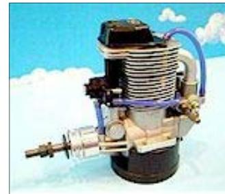
injection). He used also the new pipe (Carbon Exhaust Pipes) which is now available at Hyde Competition Products. These pipes/mufflers are made of carbon fiber and is designed for 1.20-1.40 four stroke. Price: US\$149.95. It was noticed that his model/set up is very quiet, 89dB. The engine turned a 17x12 two-blade prop at 7600-7800 RPM with 20% nitro. This prop size was also used by several OS140 RX (&FI) along with the Super Tiger 2300.
