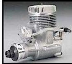
This is a side exhaust engine that comes complete with a silencer but the engine is without any fuel pump. According to OS it should deliver 3,7 hp at 9000 RPM. The weight is 925 grams. It swings props at a size of 18" or bigger according to pilots who has tested the engine.
